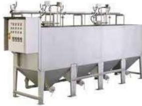
Soybean Soaking & Washing Machine use compressed air injection in water to roll the beans, separate bad Soybean and other impurities which float on the water and then are simply discharged with overflow to get the pure soybean.
