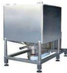
This machine is used to dissolve sugar in the soy milk in the right quantity and provides taste to the product.
