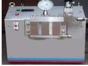
This equipment is used in the production of liquid mixtures in which the said mixture, is forced through a small passage at high velocity. This machine reduces solute globule size to a very small size in order to prevent aggregate formation.
